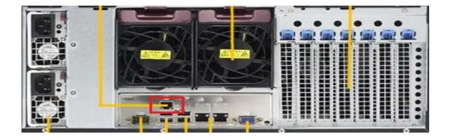
Power on the system, and press [Del] key to enter BIOS Setup Utility. Go to the [Server Mgmt] tab and select [BMC network Configuration] item.
