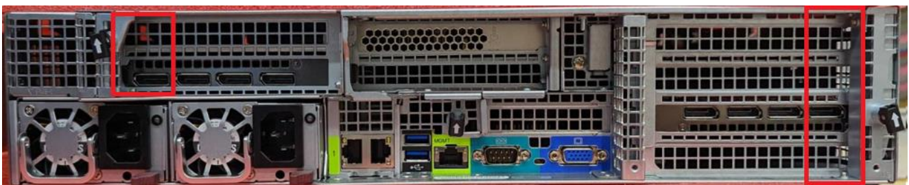
Figure 3. DP location which cannot connect to DP connector
