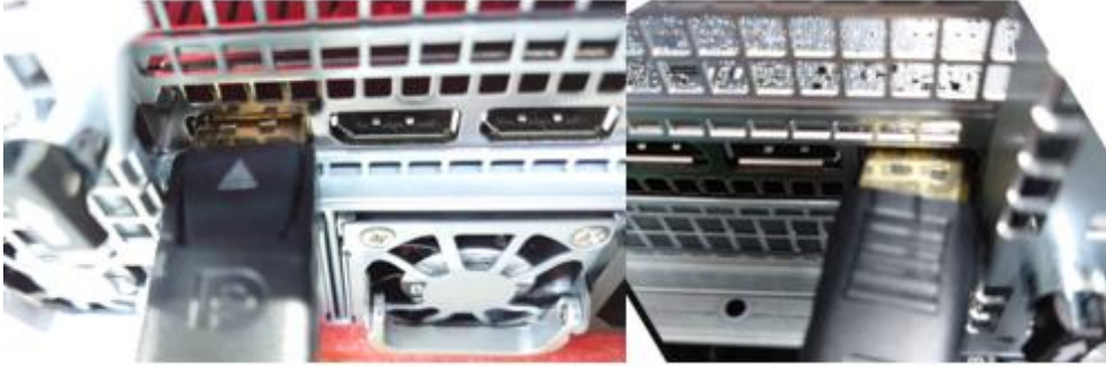
Figure 4. DP connector conflict with BrainSphere R380 F5 chassis
