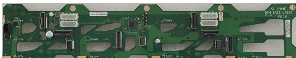
Figure 3-19. Storage Backplane BPN-SAS3-LA26A-N12 ( manual )
